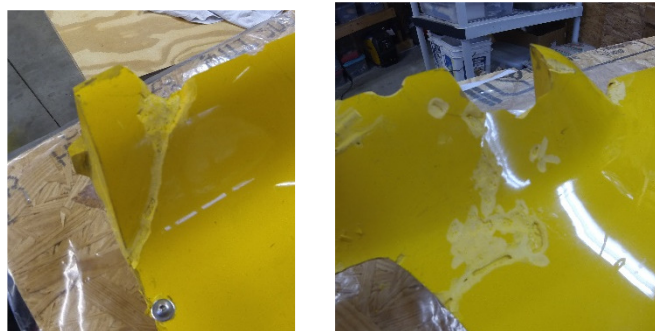
Surface Cracks and Flaws
