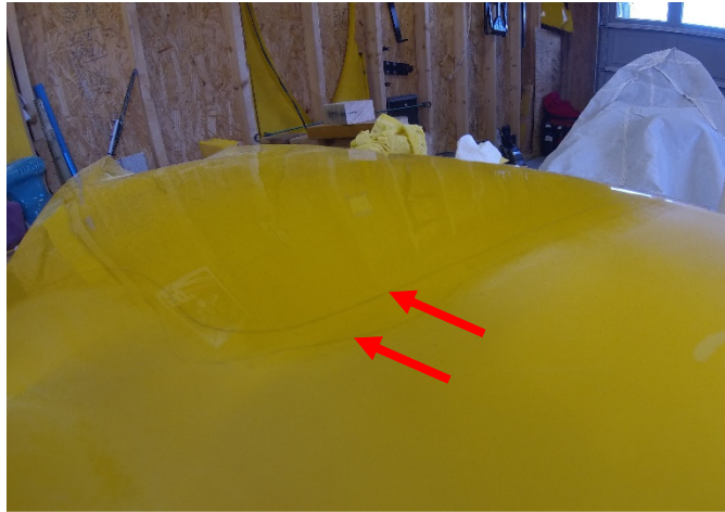
Crayon Lines used to Define Extents of Previous layer of Sanding
