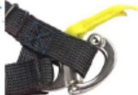
4. Counterfeit devices have electric green pull-tethers that attach to the helmet. This pull-tether resembles a shoe string rather than authentic Nomex™ thread.
