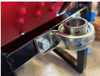
Steering was relatively straight-forward, using 2 pillow-block bearings from McMaster, a bolt-on bracket for the handlebars, and a fork fabrication left over from an earlier project.
