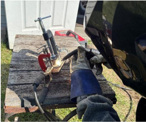
Oscar did all the welding. Impressive for his first project. I set him up for success by basing the design on 1-inch square, .080 wall thick tubing and flux-cored MIG welding. This thickness material will be resistant to burn-through and the flux-cored MIG is about as easy as welding gets. When the metal gets below ~.060, burn through can become a problem especially with MIG.
