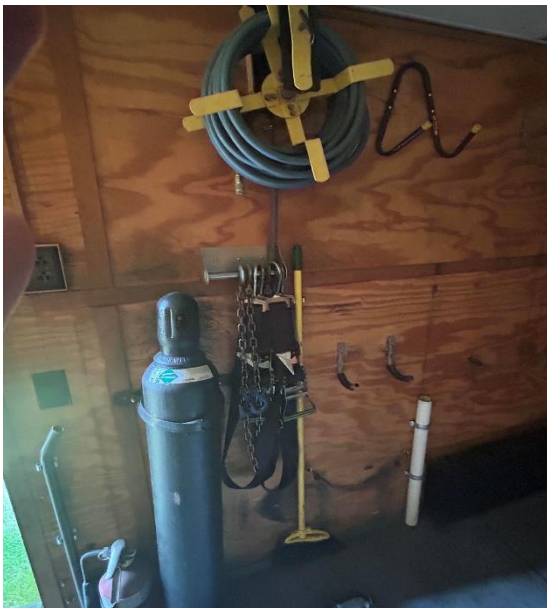
Nitrogen bottle, industrial grade regulator, mounting bracket and 25 ft. air hose with reel.
